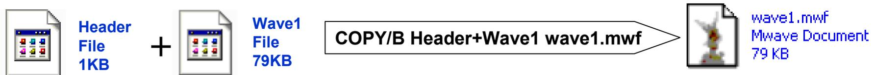
MFER defines as a gathering on a frame which consist of header and waveform. Header is described with sampling attributes, waveform frame attributes and other supplemental information.
